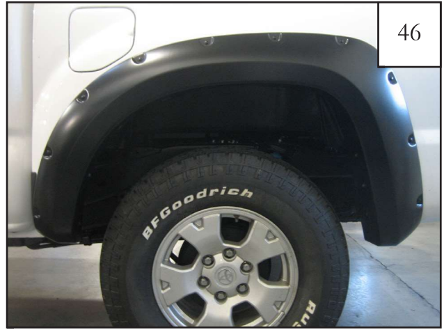
Completed rear flare installation.
