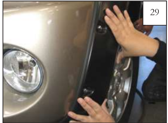
Situate flare on bumper, inserting screws through holes drilled in bumper in step 26.
