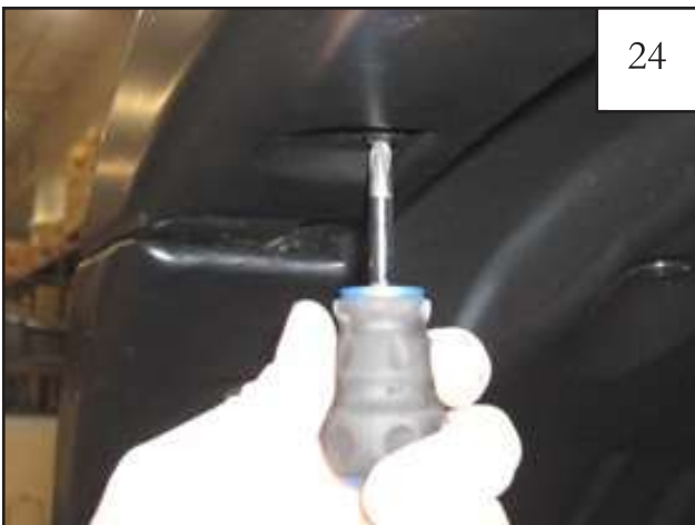
Install a supplied Screw (SW1-0050) through hole in flare and into Clip installed in step 22. 4 places.
