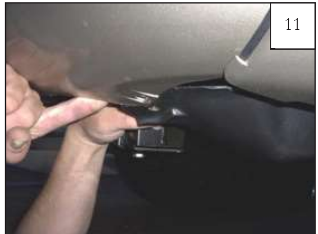
Pull down bumper cover and splash shield.
